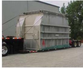
*Modular collecting section for a Tubular Up-Flow WESP*
